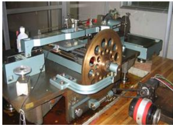
Fig.14. Grating ruling machine
