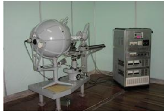
Fig10. Stray light tester
